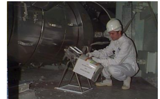
EMECC measurement of a hot leg of a PWR RCS
