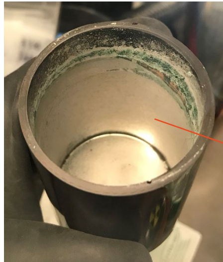
After the 2 m/s Test using thermally purified salt
