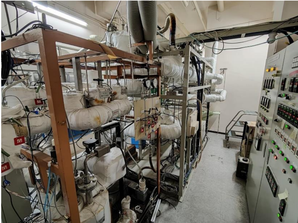
FIG.1. Existing LiPb test loop at Kyoto University.
