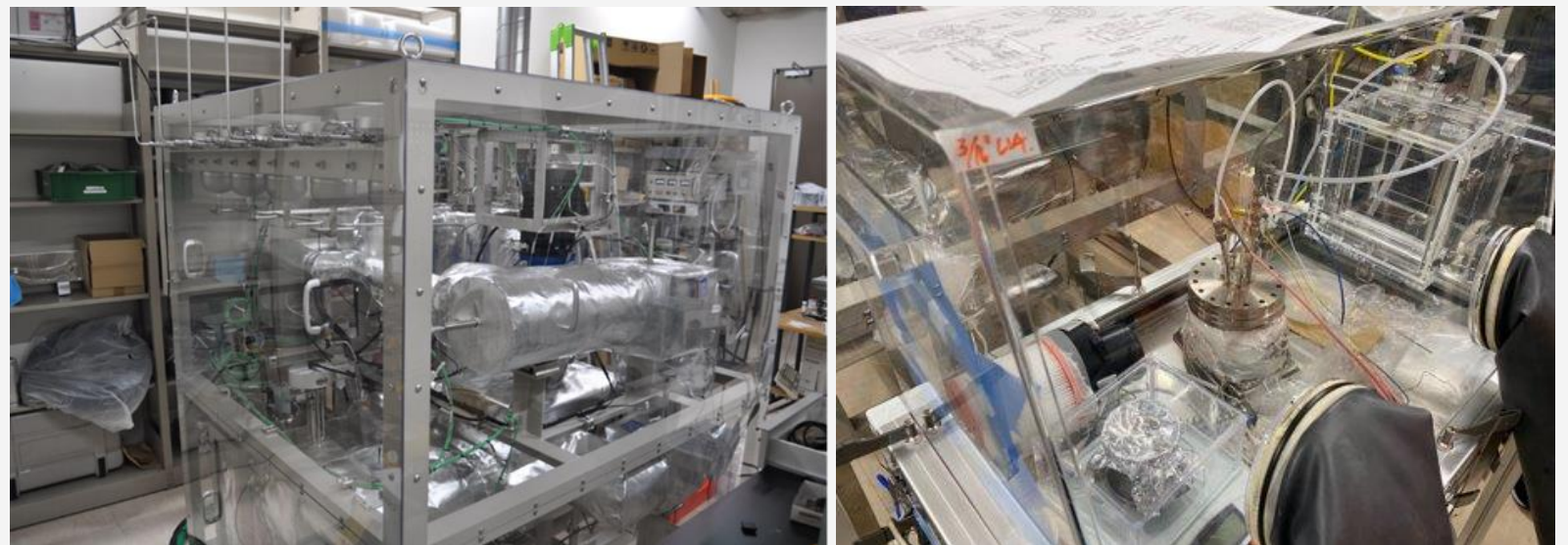
FLiBe Loop (left), FLiBe Purification Glovebox (right)
