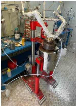
FIG. 1. Autoclave (2.5 l) of the experimental loop.
