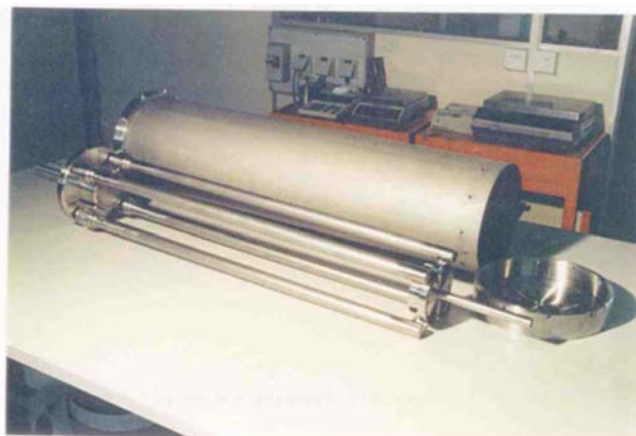
FIG. 3. PRIAM process for the Cold Trap regeneration [20].
