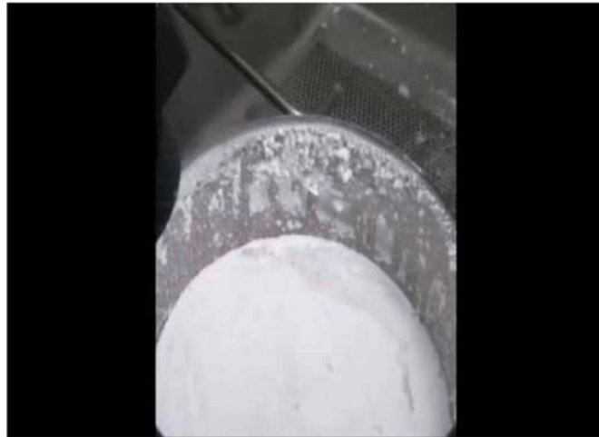
FIG. 5. Carbonation process: sodium converted into sodium carbonate.
