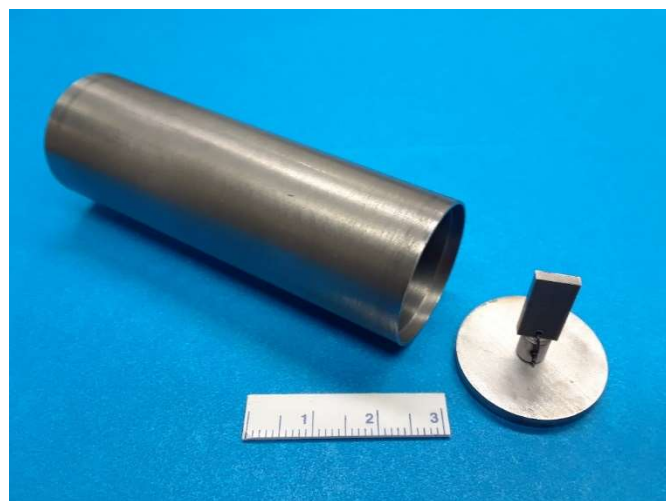
FIG. 2. An open molybdenum capsule with a corrosion coupon attached to one lid. The capsule is filled with salt, welded shut, and then sealed within a stainless-steel outer capsule. The scale shown in the image is in cm.
