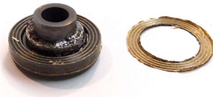
FIG. 5. The seal after the test.
