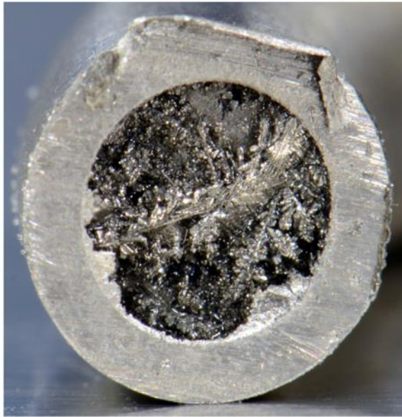
Kelleher 2022 Materials Today - Ni 200 loop, 14 h at 620°C, unpurified NaCl-MgCl 2 salt
