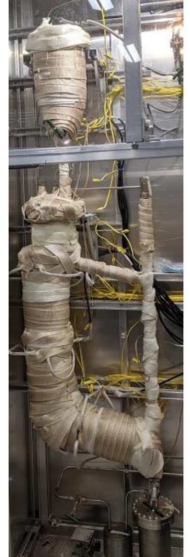
Thermal convection loop
