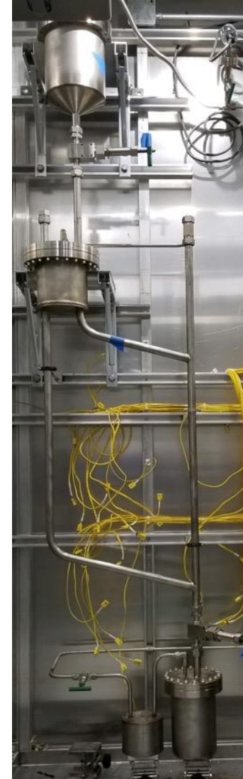
Thermal convection loop
