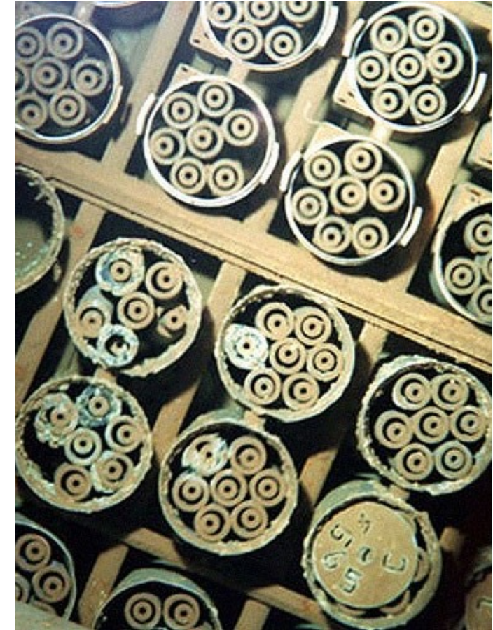
Spent nuclear fuel stored underwater and uncapped at the Hanford site
