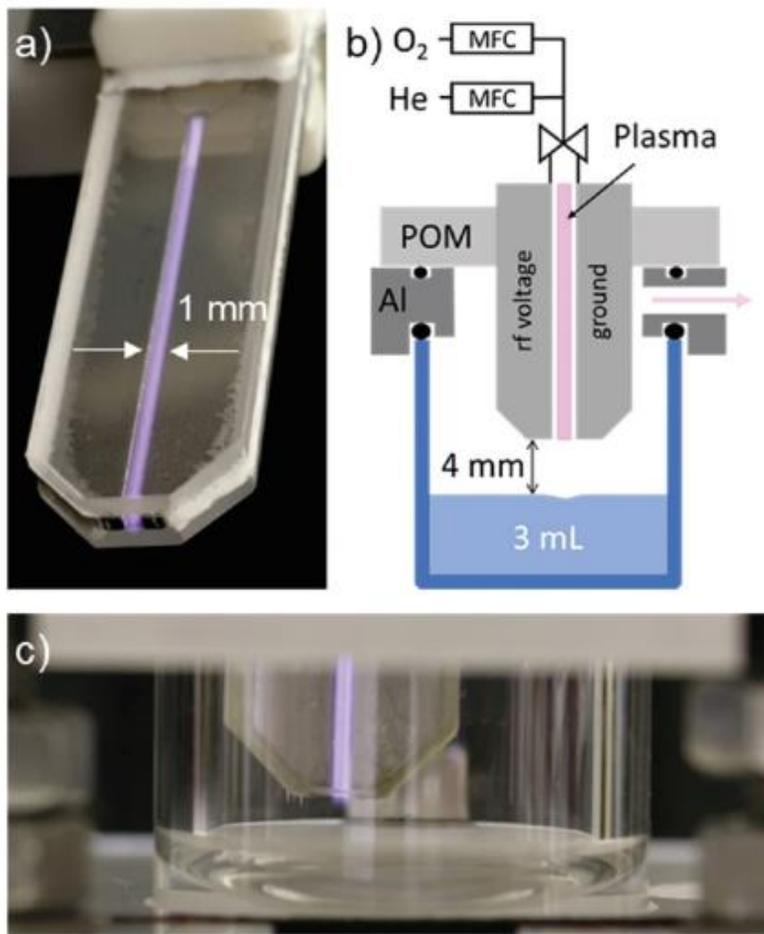
He + <1% of molecular gas (O<sub>2</sub>, H<sub>2</sub>O, N<sub>2</sub>,...), RF driven 13.56 MHz at 230 Vrms
