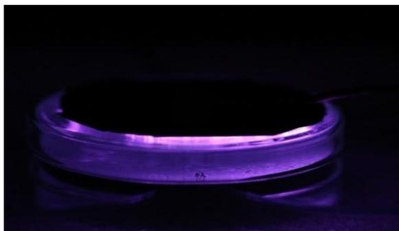
glass Petri dish covered by aluminium foil as DBD electrodes: (d=100mm, l=2mm)
