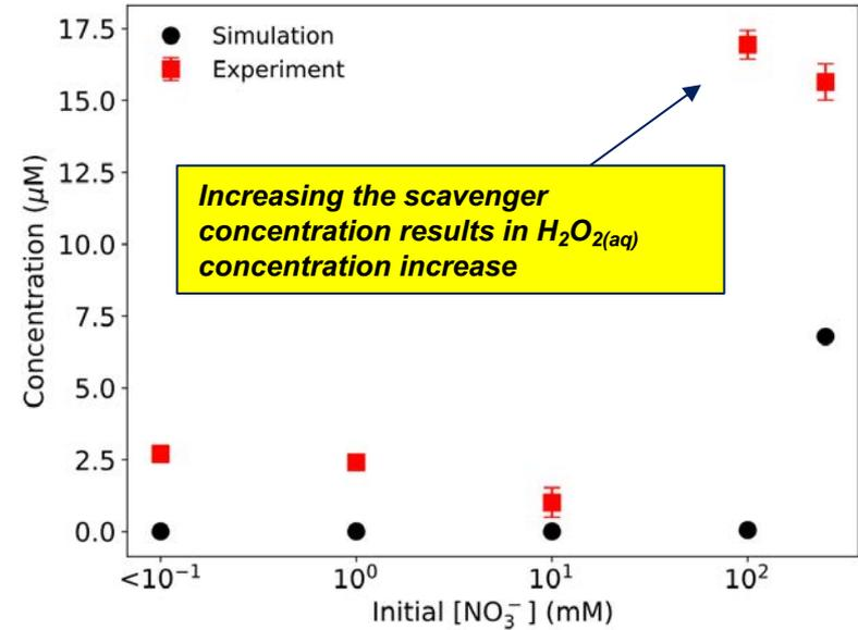
Experimental measurements of hydrogen peroxide concentration as a function of initial  $\text{NO}_3^-_{(aq)}$  concentration added to the solution. Increasing the scavenger concentration from 10 to 100 mM results in  $\text{H}_2\text{O}_{2(aq)}$  concentration increase from around 2.5 to 17  $\mu\text{M}$ . Additional  $\text{NO}_3^-_{(aq)}$  beyond 100 mM slightly decreases  $[\text{H}_2\text{O}_{2(aq)}]$ .
