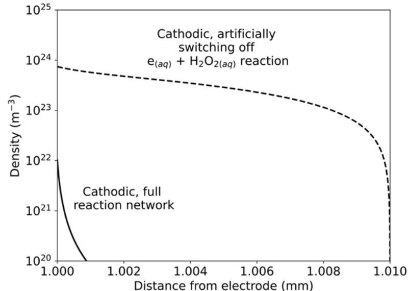
*Aqueous hydrogen peroxide concentration at steady state in the cathodic case. The dotted line shows the concentration in the cathodic case with the reaction with solvated electrons switched off,*
