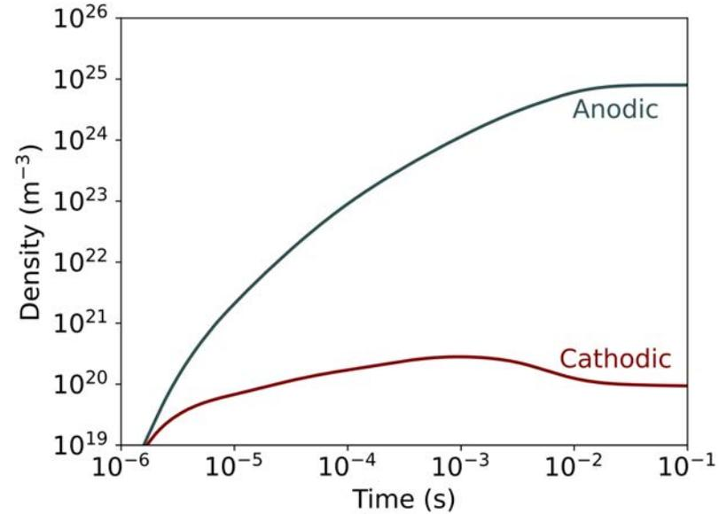
*Average concentration of  $H_2O_{2(aq)}$  over time in the  $10 \mu m$  liquid film. In both cases  $H_2O_{2(aq)}$  reaches steady state after  $\sim 10$  ms, but in the anodic case the average value is over **4 orders of magnitude larger**.*
