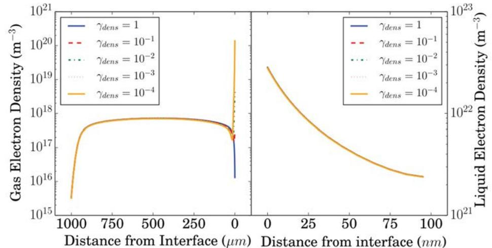
Electron density as a function of interfacial loss coefficient in the gas phase (left) and water phase (right). Simulation was performed with Zapdos. Figure adapted from [4].
