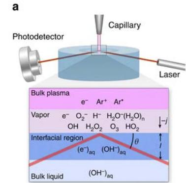
Top: NO<sub>2</sub><sup>-</sup> production in a plasma-water reactor. [1]
