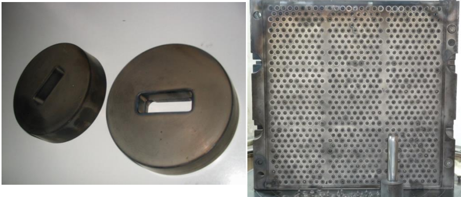
Plasma nitrided die for manufacturing bottle top lid (D2 material), extrusion dies (H13), Wash basin (Inconel 600)
