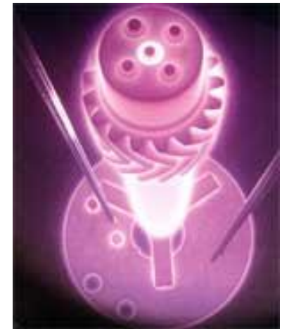
Plasma glow around components; Note the uniform plasma covering the component
