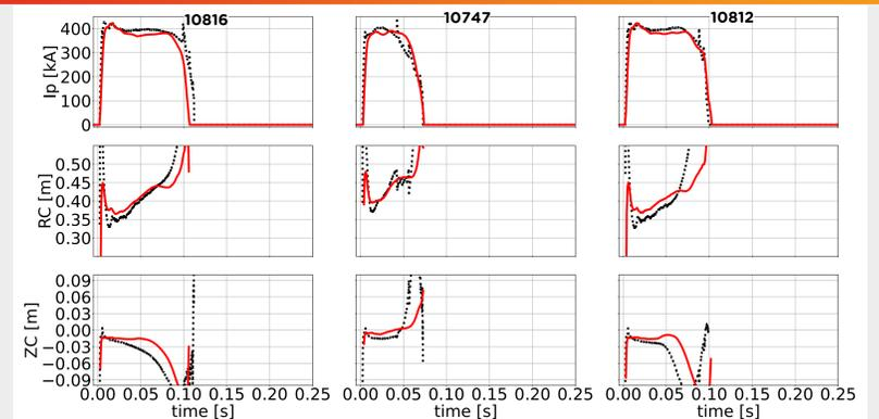
Experiments 10816, 10747, 10812. Top to bottom: Plasma current, radial and vertical centroid positions. Dotted/solid lines: reconstruction from experiment/prediction.
