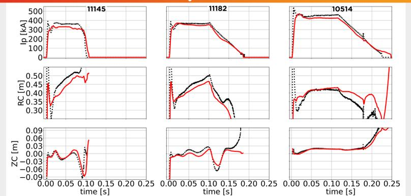
Experiments 11145, 11182, 10514. Top to bottom: Plasma current, radial and vertical centroid positions. Dotted black/solid red lines: reconstruction from experiment/prediction.
