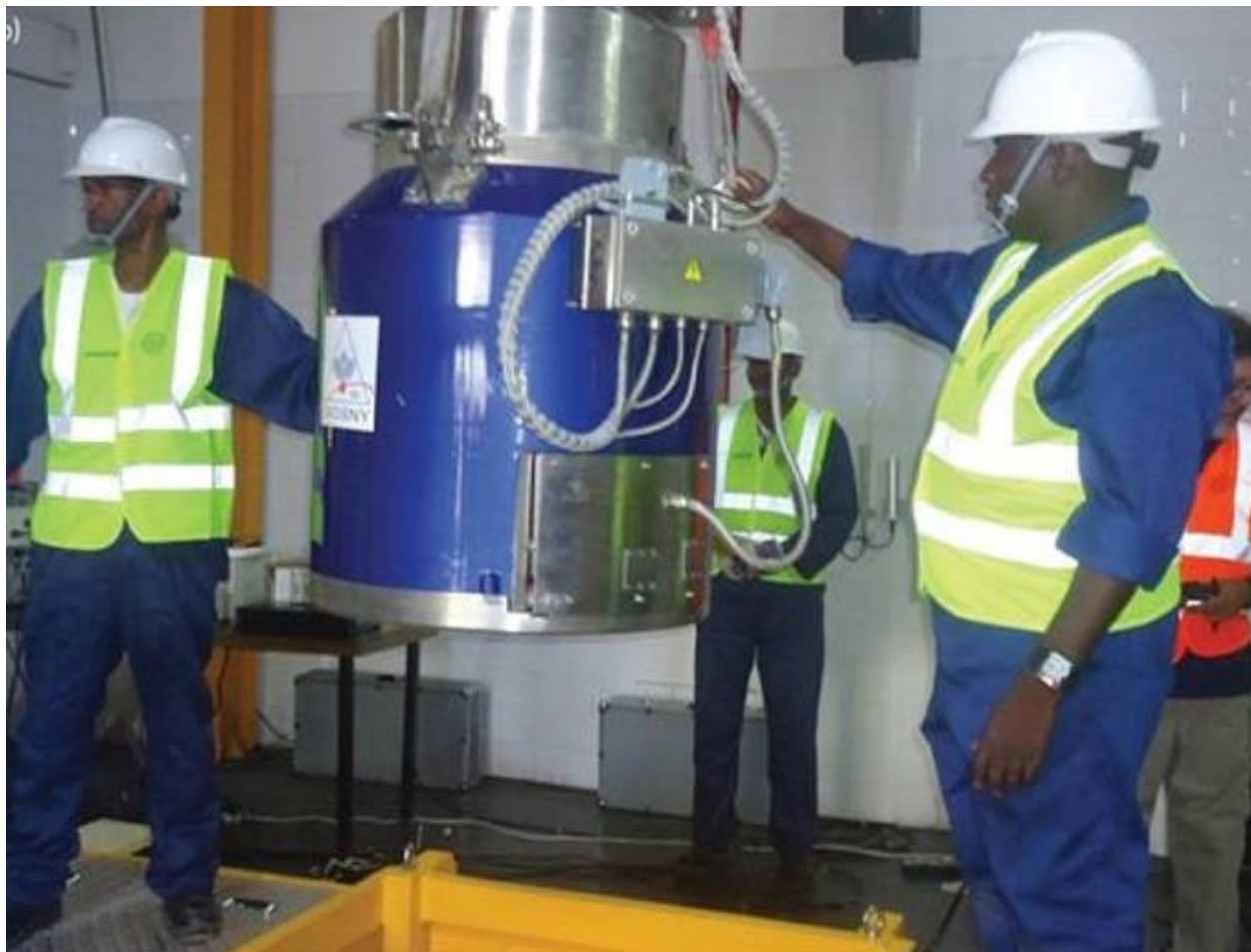
Fig. 1. CERT Engineers and Technicians Lifting an Interim Transfer Cask with HEU Spent Fuel [2]
