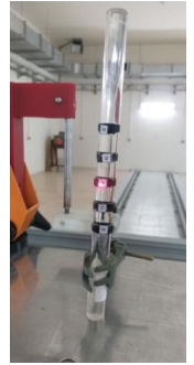
Ring dosimeters are fixed on rod phantom for calibration
