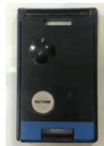
Harshaw TLD reader 4500 with WinRems software (left), Harshaw TLD with two chips TLD-100 for measuring \text{Hp}(10) and \text{Hp}(0.07) (right)
