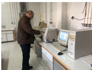
Harshaw TLD reader 4500 with WinRems software (left), Harshaw TLD with two chips TLD-100 for measuring \text{Hp}(10) and \text{Hp}(0.07) (right)
