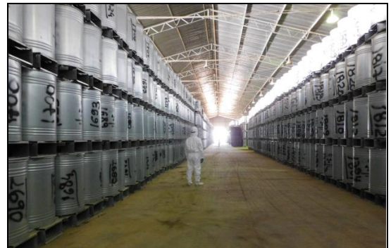
Figure 4. Overpacked drums on new steel pallets in the Shed C-05.
