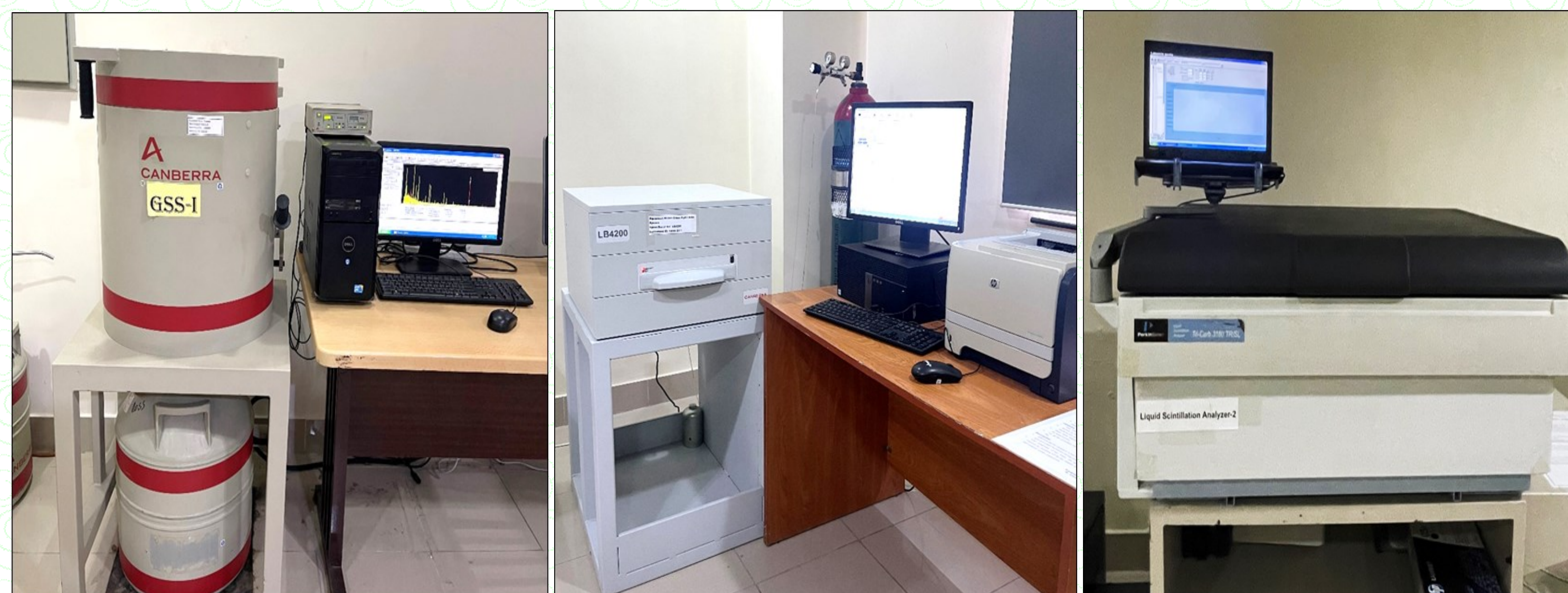
Fig.02. (From L to R) Gamma Spectrometry System, Gross Alpha beta Counting System, Liquid Scintillation Analyzer
