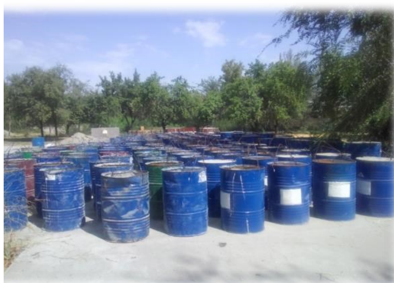
200 l drums with radioactive wastes
