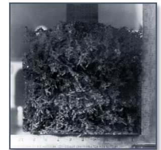
Uranium recovered from EBR-II fuel
