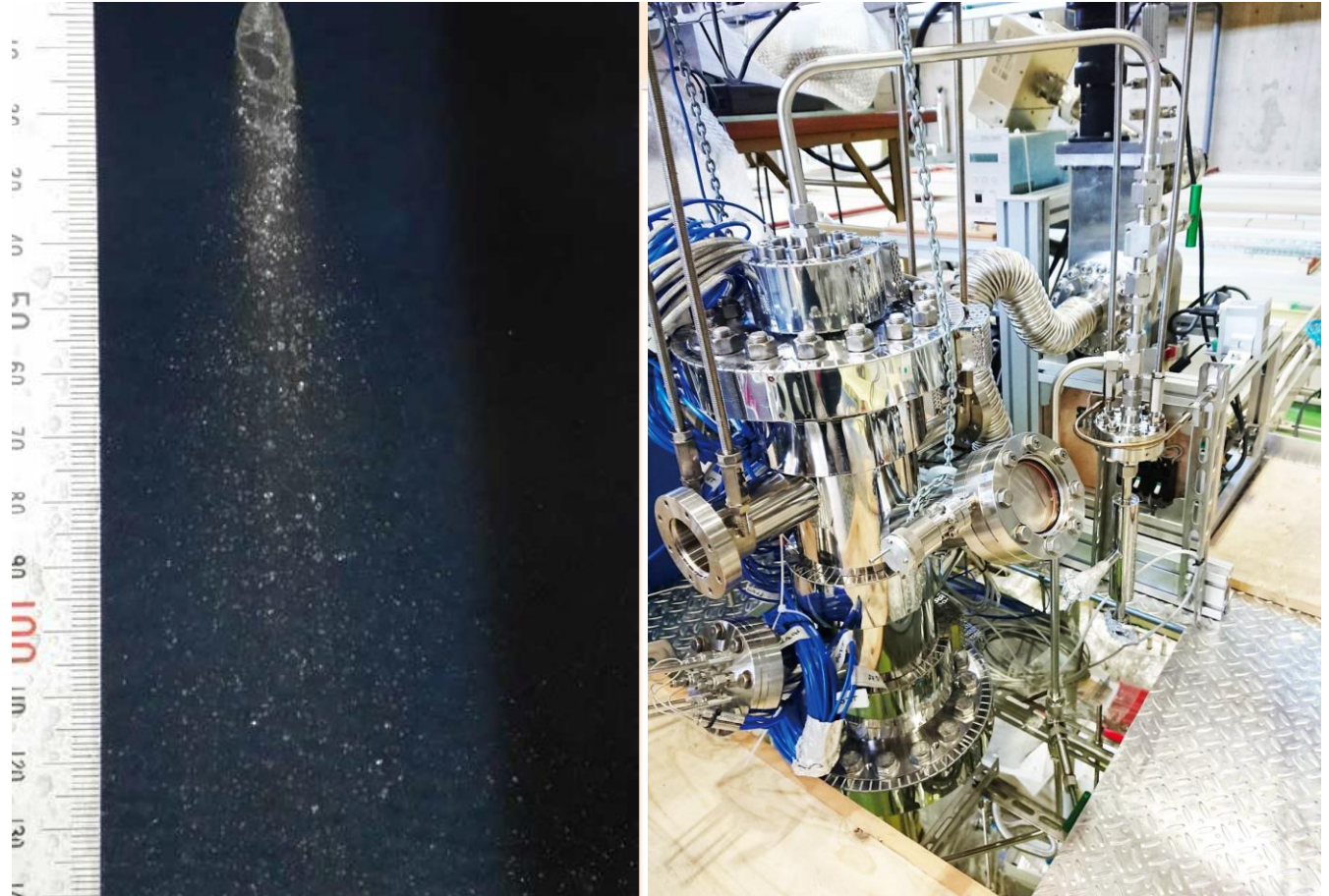
Tritium extraction demonstration from LiPb Loop via Vacuum Sieve Tray
