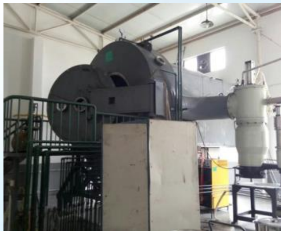
Fabrication facility of Be pebbles based on rotating electrode method @SWIP & HaiBao
