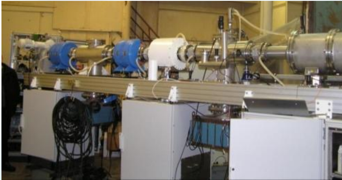
D-T neutron sources ( \sim 10^{11}\text{s}^{-1} ) (@CAEP)
