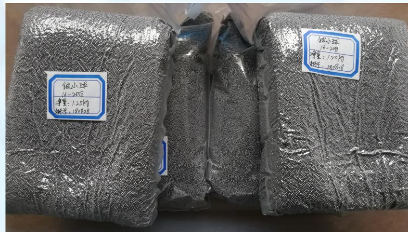
Beryllium pebbles fabricated by 10kg / batch process
