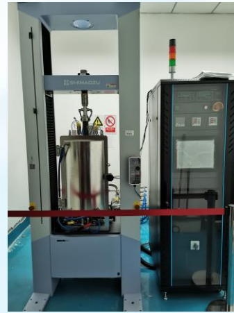
Thermal mechanical with compress load
