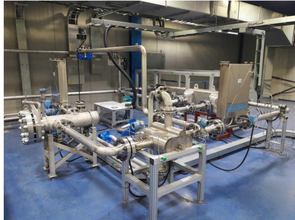
Helium Supply System (HeSS) for HCCR TBS HCS performance test
