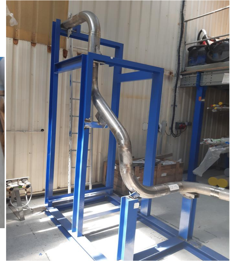
View of the mock-up of the guard pipe + process pipes manufactured in 2021
