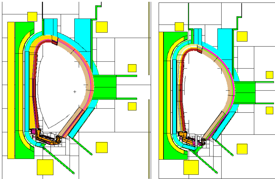
Figure 4 EU DEMO MCNP model with HCPB (left) and WCLL (right) blanket concept
