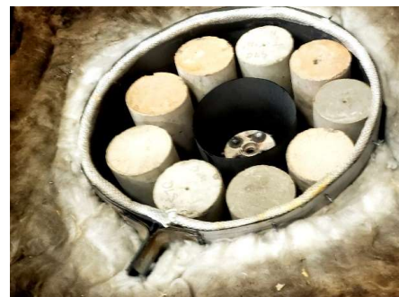
Concrete Heated to 350 to 800 F (177 C – 427 C)
