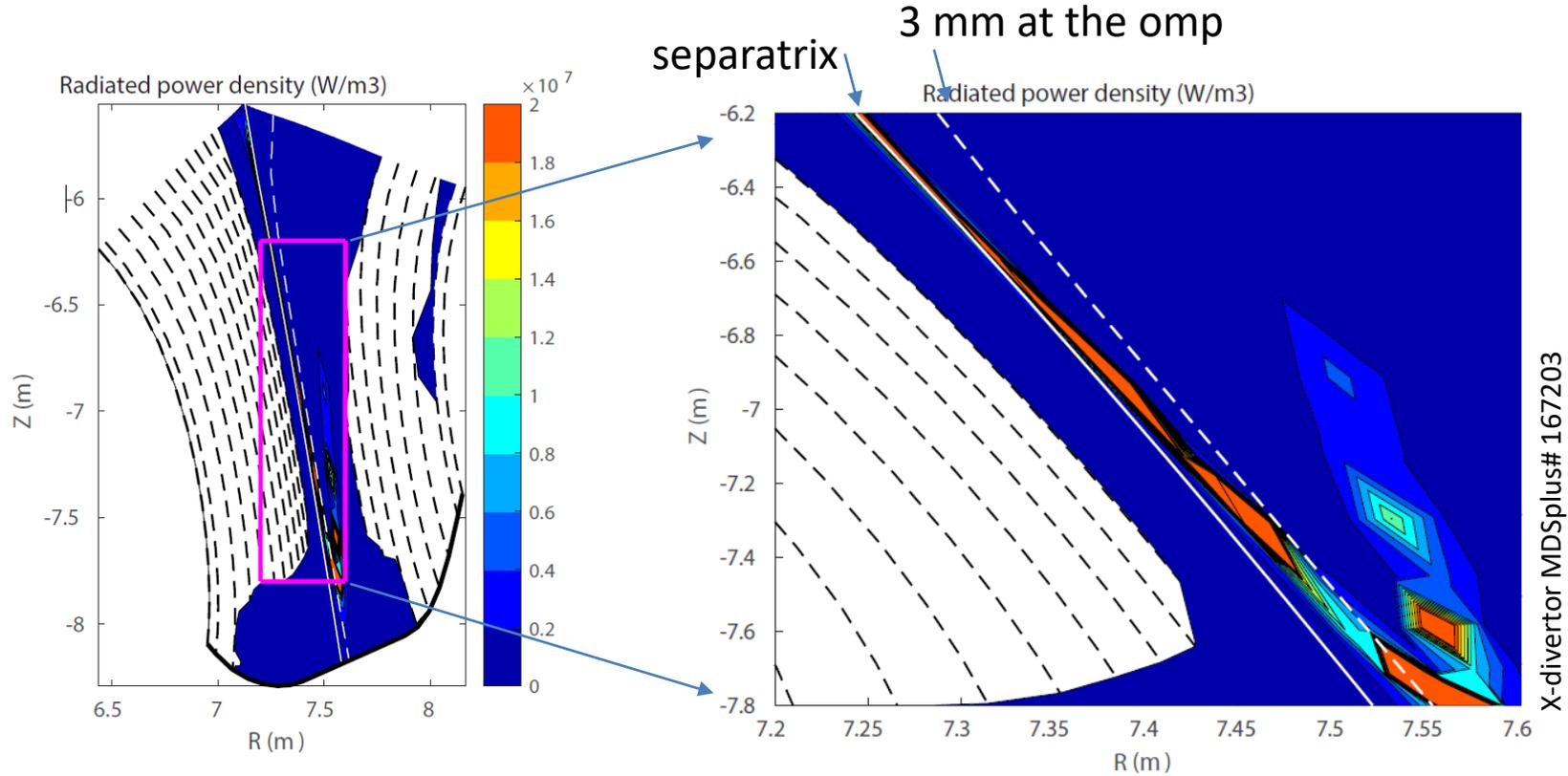
The end result is strong argon radiation in relatively low  $T_e$  regions, without a Lengyel model like collapse of  $T_e$
