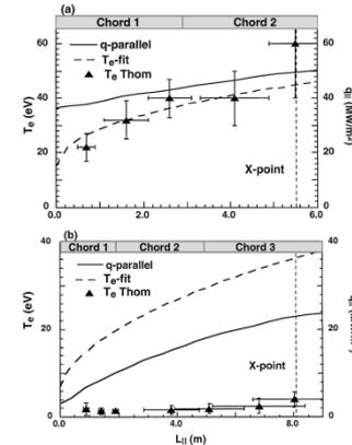
FIG. 2. The outboard divertor energy flux analysis for (a) standard ELMing H mode and (b) radiative divertor through deuterium puffing. Shown are the energy flux profile,  $q_{||}$ , the fitted  $T_e$  profile for conduction dominated transport, and measurements of  $T_e$  from divertor Thomson scattering measurements. Shown at the top of the graphs are the approximate view locations of the horizontal viewing bolometer chords.
