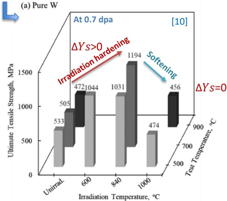
Softening under neutron irradiation leads to reduce the irradiation-enhanced embrittlement of tungsten
