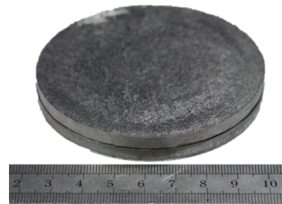
Component design, W f /W joint with steel via V 20 mm to 105 mm in diameter
