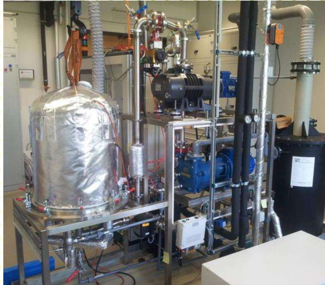
WILMA: W Infiltration Machine Setup for the chemical deposition of W installed at Forschungszentrum Jülich [Riesch et al., Nuclear Materials and Energy 9 (2016) S. 75–83]
