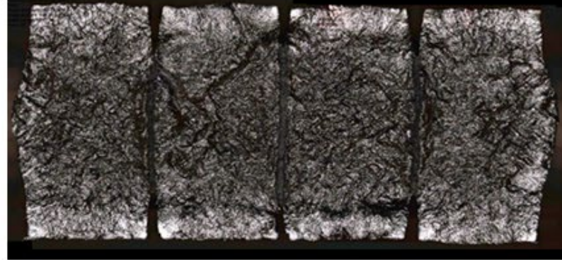
25 MW/m 2 , 1000 cycles (Coolant: 105 °C)
