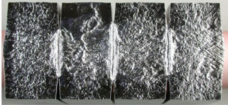
25 MW/m 2 , 500 cycles (Coolant: 105 °C)
