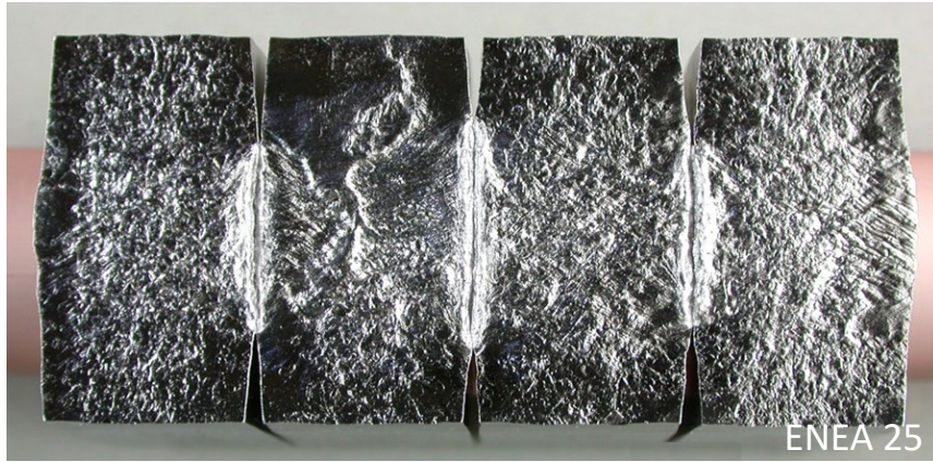
Surface roughening due to deformation
