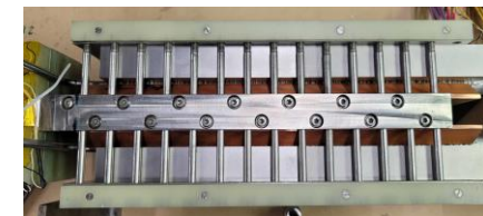
Benchtop-scale superconducting joints that have been fabricated for ARC magnets
