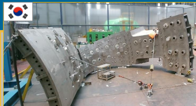
Vacuum Vessel Sector Assembly
