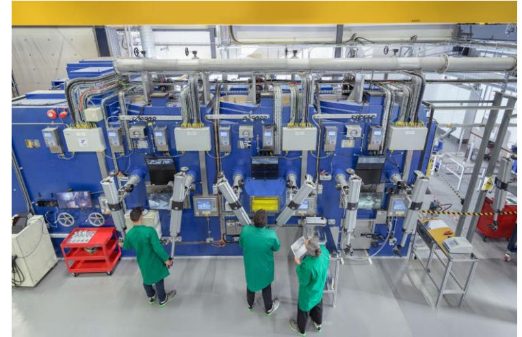
UKAEA's Materials Research Facility (MRF) prepares and examines samples of radioactive materials to assess their performance © UKAEA
