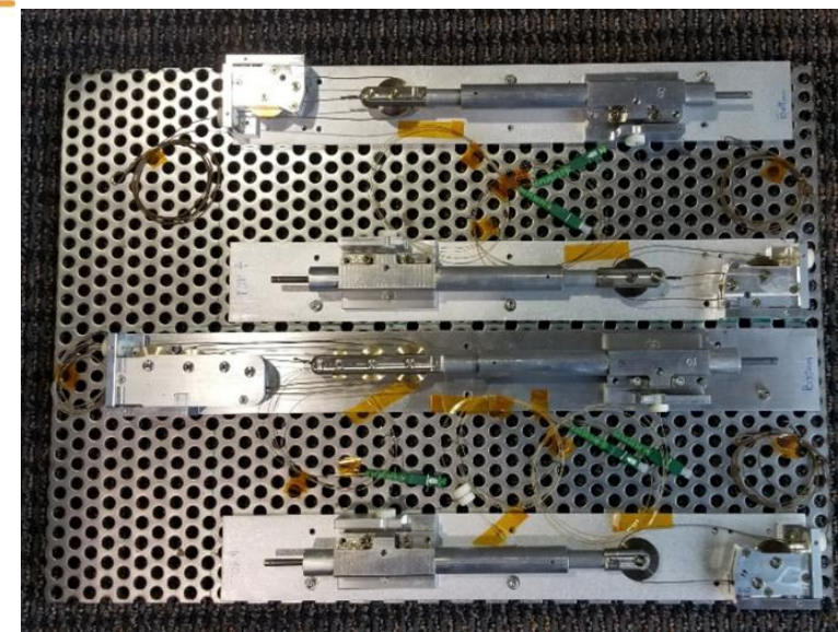
Sensors and NiCr metallic wire
