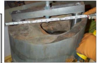
Nozzle #3 Area Cut Away From Reactor Head
