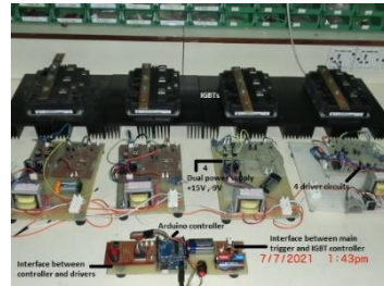
IGBT gate drive controller
