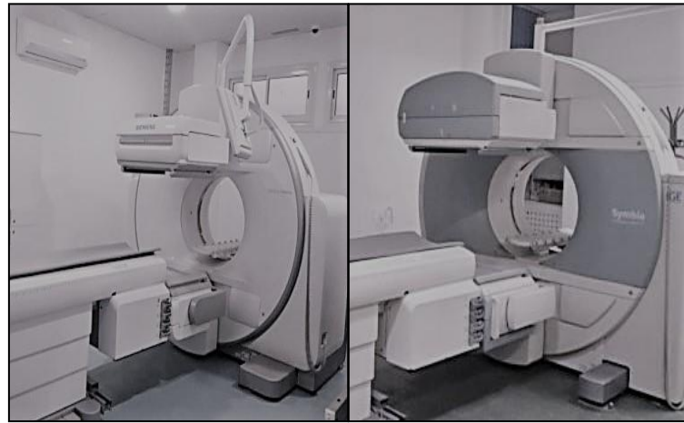
Figure 1: Our nuclear medicine department equipped with Gamma Cameras integrated SPECT and CT System
