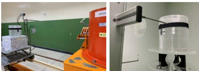
FIG 2. Irradiation of ^{137}\text{Cs} (left) and ^{90}\text{Sr}/^{90}\text{Y} sources (right) to nanodot dosimeters in term of eye lens dose.
