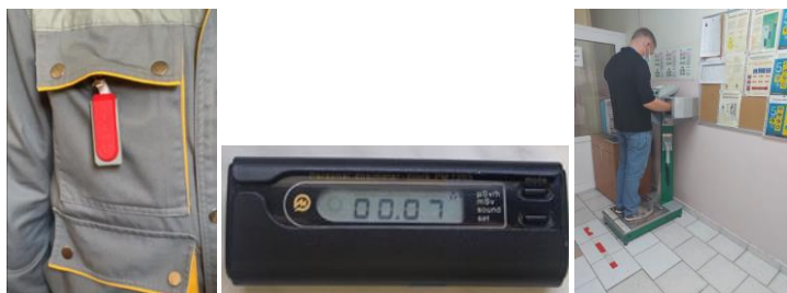
The main methods of individual monitoring are thermoluminescent dosimeters, personal dosimeters as well as the use of computational methods
