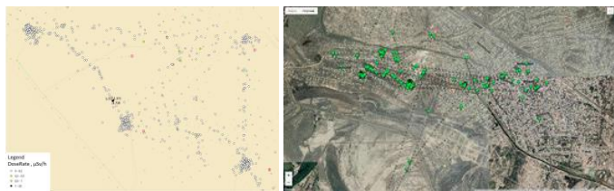
Examples of gamma-ray surveys of a wellfield and the territory of a settlement located near the production sites
