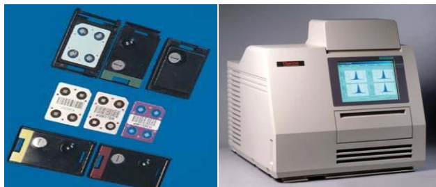
Fig 2: Harshaw 6600 Plus TLD Reader
