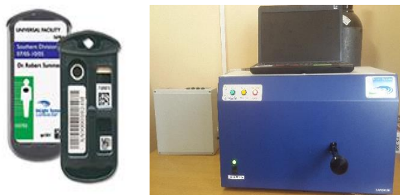
Fig 1: Landauer Semi-Manual InLight OSL Reader
