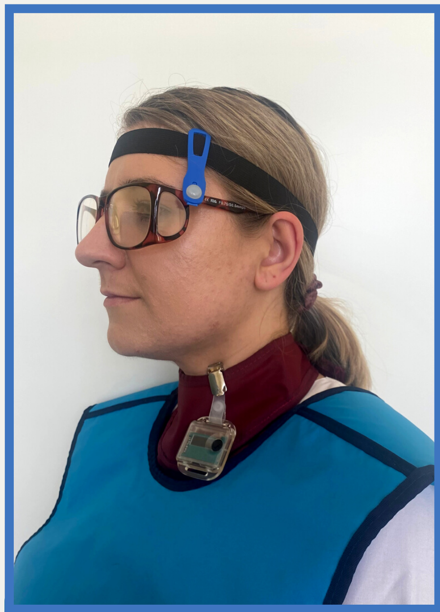
Figure 1. The dose to the lens of the eye can be assessed by measuring personal dose equivalent H_p(3) with the eye lens dosimeter at the level of the eye or H_p(10) with the whole body dosimeter above the lead collar in Lithuanian hospitals.
