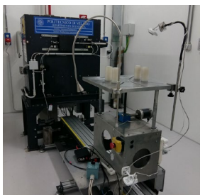
Self-shielded gamma irradiator (left) and X-ray generator (right) hosted in the ionizing radiation laboratory of the LMR
