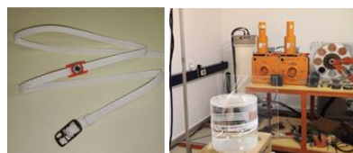
Figure 1. Left: H_p(3) dosimeter assembled Right: dosimeters allocated in water phantom for irradiation
