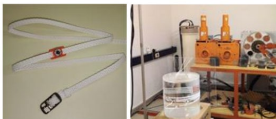
Figure 1. Left: Hp(3) dosimeter assembled Right: dosimeters located in water phantom for irradiation
