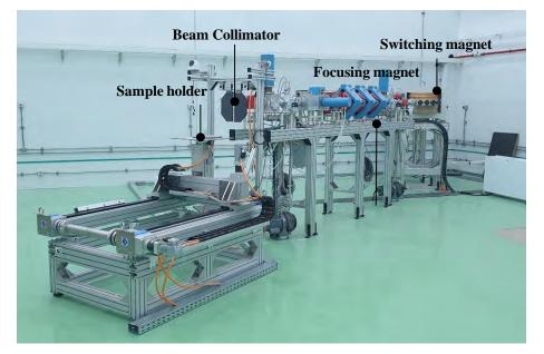
FIG. 1. The current setup of R&D beam line consists of a five-port switching magnet, a set of quadrupole magnets and a graphite collimator mounted at the end of the horizontal beam line.
