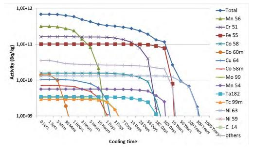
Figure 1. Time evolution of activity induced in the TC liner
