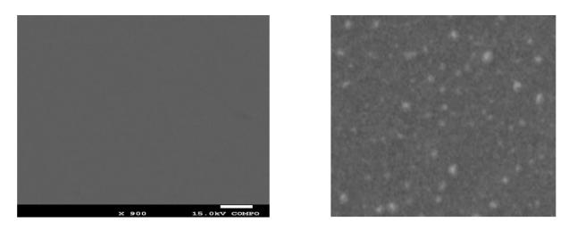
FIG.1. SEM images of a implanted TiO2 film before (left) and after annealing (right) at 500 °C, 15 min.
