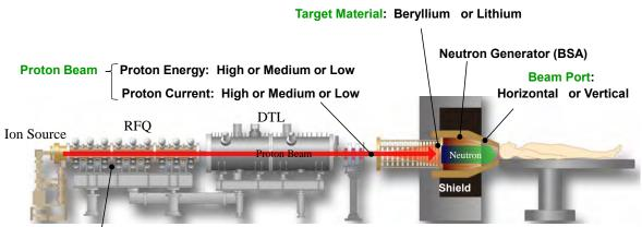
Proton Accelerator: Cyclotron or Linac or Electrostatic
