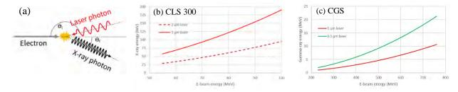
FIG. 1. (a) Principle of inverse Compton scattering. (b) X-ray and (c) gamma-ray energy as a function of electron energy.
