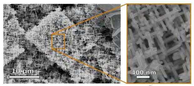
Fig. 1 SEM image of a Bi nanowire network consisting of  $1.4 \times 10^9$  wires per cm<sup>2</sup> with a wire diameter of ~100 nm together with a close-up illustrating the wires interconnected within the network.
