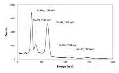
FIG. 1. NaI gamma spectrum of Mo / Tc isotopes generated from the irradiation of a natural Mo target during [<sup>18</sup>F]FDG manufacturing
