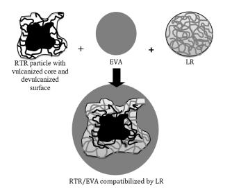
FIG 1 Schematic representation of RTR/EVA blend compatibilization by LR
