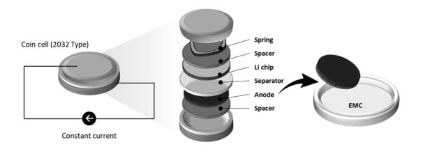
FIG. 1. Sample preparation/lithiation in a coin cell setup for later post-mortem analysis through IBA.
