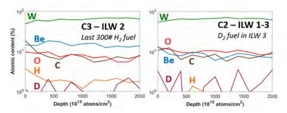
FIG. 1. HI-ERDA depth profiles of elemental composition on W samples from neighbouring positions C3 and C2, retrieved after ILW-2, which finished off with 300 shots of H2, and ILW-3, which finished with D2 fuelling. The total hydrogen isotope retention is  $6.7 \times 10^{16}$  and  $5.3 \times 10^{16}$  cm<sup>-2</sup>, respectively.
