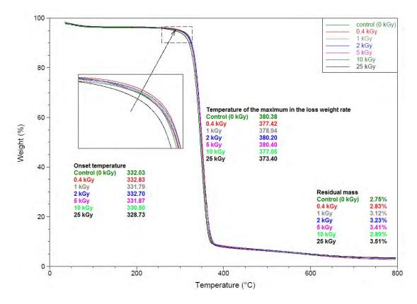
FIG. 1. TGA curve for thermal decomposition of Whatman CHR1 paper.
