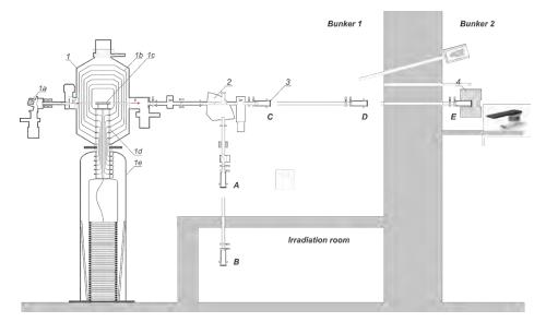
FIG. 1. Layout of the experimental facility: 1 – vacuum-insulated tandem accelerator (1a – negative ion source, 1b – intermediate- and high-voltage electrodes, 1c – gas stripper, 1d – feedthrough insulator, 1e – high-voltage power supply), 2 – bending magnet, 3 – lithium target, 4 – beam-shaping assembly. A, B, C, D, E – lithium target placement positions.
