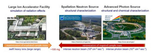
FIG. 1. Swift heavy ions with large penetration depths are required to produce sufficiently large quantities of homogeneously irradiated materials (~100 mg) that can be analysed by spallation neutron and synchrotron X-ray probes.
