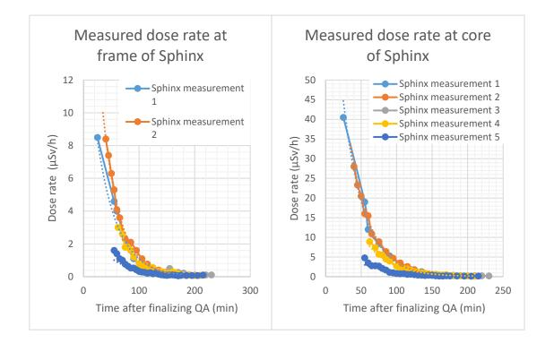
Spectrum-based measurements performed on activated metallic parts of the accelerator show the presence of Co-57 and Co-60. Dose rates at contact can vary significantly, from a few  $\mu$ Sv/h up to 1 mSv/h for the most activated components.
