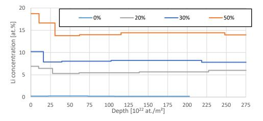
FIG 2: Comparison of the Li depth profiles. The first ~6  $\mu$ m are enriched with Li. The region >200\*10<sup>22</sup> at./m<sup>2</sup> has to be considered with care due to the dominance of the pile-up signal in this deep region.
