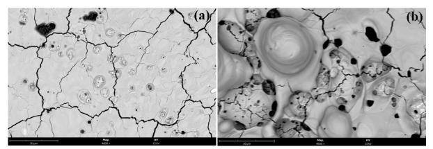
FIG. 1: SEM images of (a)  $W_{20}Ta_{20}Cr_{20}Nb_{20}V_{20}$  and (b)  $W_{30}Ta_{17.5}Cr_{17.5}Nb_{17.5}V_{17.5}$  after 3 discharges.
