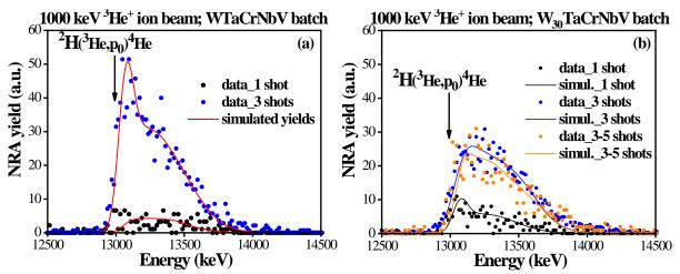
FIG. 2: NRA spectra and corresponding fit lines achieved from the elemental quantification using the NDF code [6]: (a)  $W_{20}Ta_{20}Cr_{20}Nb_{20}V_{20}$  and (b)  $W_{30}Ta_{17.5}Cr_{17.5}Nb_{17.5}V_{17.5}$  alloy.
