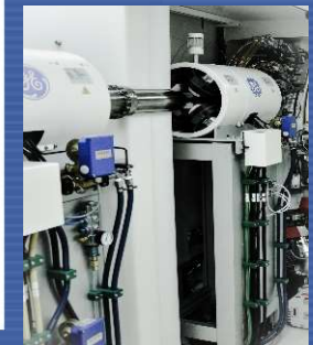
Liquid Zn target for direct production of ^{68}\text{Ga}
