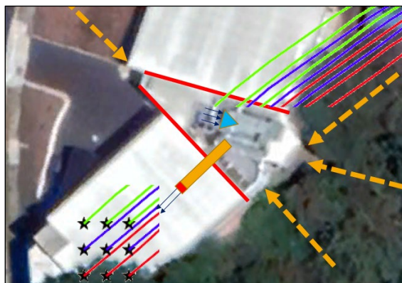
FIG. 5. Inlet (blue triangle) and exhaust pipe (orange-red rectangle) representations for change proposal with an over-position representation of the modelled wind direction, at the day and time where the recirculation incident took place.
