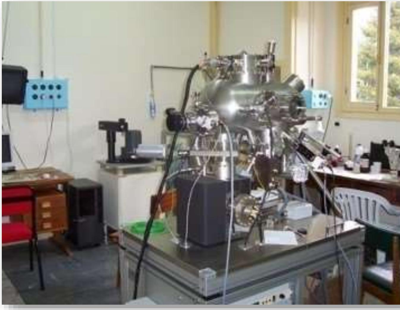
Omicron VT AFM 25 DRH microscope
