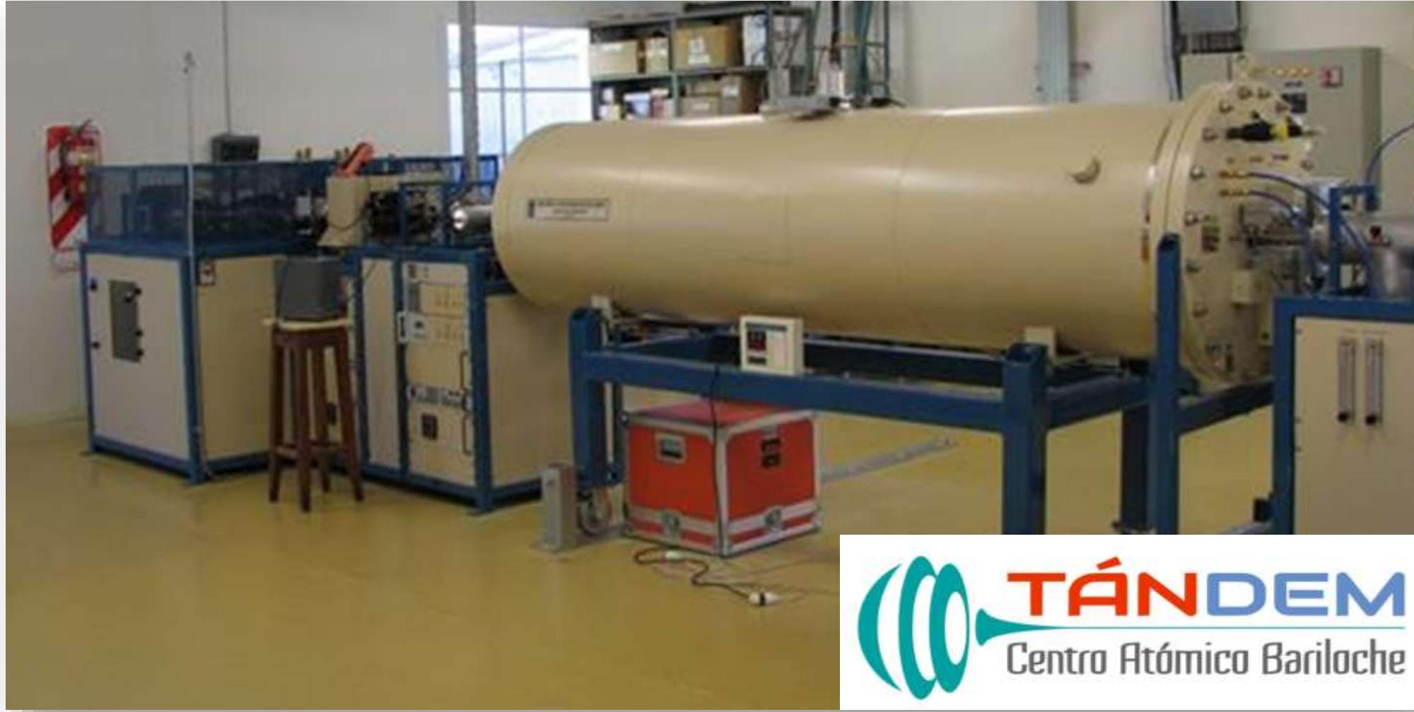
5 SDH Tandem accelerator from the National Electrostatics Corp. (NEC)
