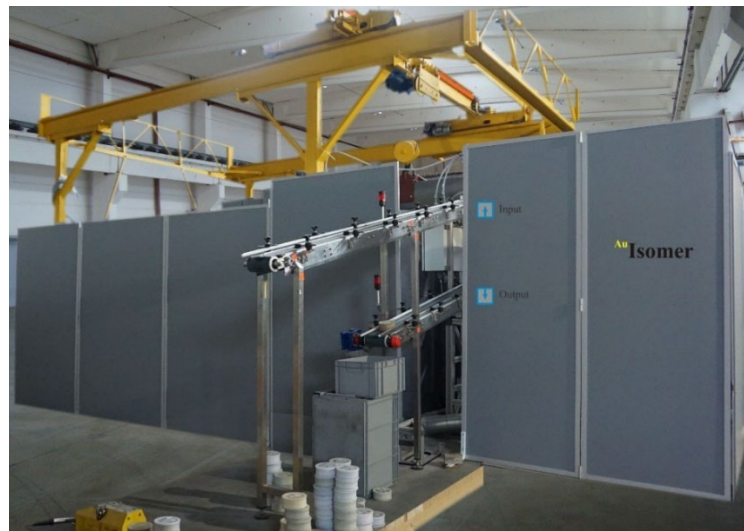
FIG. 1. "Au-Isomer" gamma-activation analysis facility.
