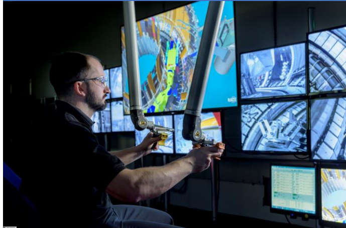
Component removal using remote handling
