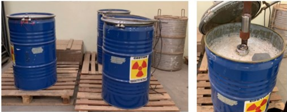
Fig. 5. Concrete drum containing conditioned sources
