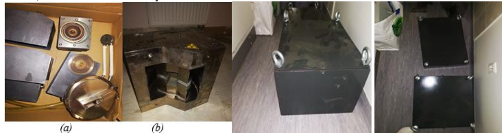
Fig.1 Activated linac parts, vacuum window of the accelerating wave-guide, the target and the flattening filter (a), bending magnet core (b)
